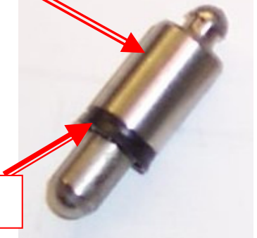
Lubricate Piston Seal with synthetic grease
